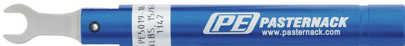
2. The PE5019-16 torque wrench for 1.0-mm connectors is a break-over type of wrench, which eliminates the possibility of over-torquing the connector.
