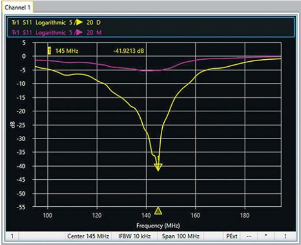
10. In this example, the unmatched antenna (purple) is only achieving 4 to 5 dB return loss, resulting in as much as 30% to 40% of reflected power. The fully matched antenna (yellow) is achieving greater than 40 dB return loss, indicating a reflected power of less than 1%.
